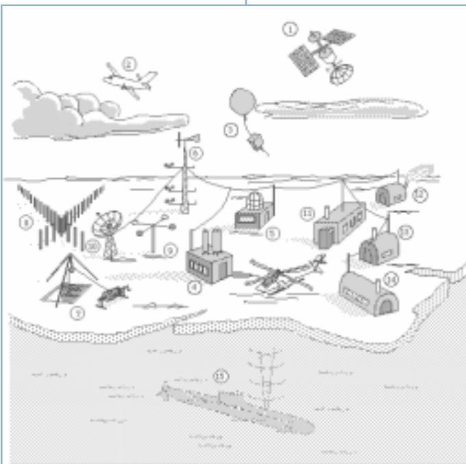
Figure 18. A sketch, made during the planning phase, of elements of the SHEBA research camp on the pack ice. The camp, which headquarters about 25 people at a time, has been deployed in the pack ice of the eastern Beaufort Sea; changes in ice conditions and leads regularly affect the actual layout. (1) Satellite for monitoring atmospheric structure and surface parameters; (2) research aircraft for surveys of atmospheric and surface parameters; (3) rawinsonde; (4) instrumentation to measure the spectral distribution of downwelling radiation; (5) all-sky camera, ceilometer, and other instrumentation to measure cloud properties; (6) meteorological tower; (7) hydrohole and winch for deployment/recovery of suspended oceanographic instruments and AUVs; (8) stakes representing the measurement of the ice and snow mass balance, and temperature and radiation in the ice interior; (9) radiometers; (10) communications antenna; (11) mess hall; (12) generator shed; (13) living quarters; (14) laboratory; (15) submarine for surveying the ice thickness distribution. Figure provided by Norbert Untersteiner.
