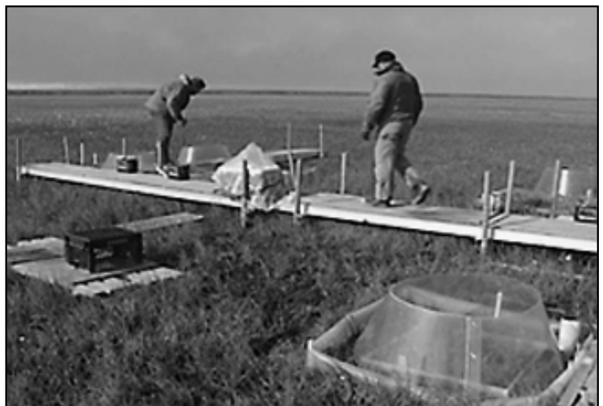
Rommel Zulueta and Rob Richardson from San Diego State University determine the effects of alteration in temperature and soil water status on net ecosystem \text{CO}_2 flux in the coastal tundra at West Dock (within the Prudhoe Bay, Alaska oil field) in 1996. The water table was manipulated by float-activated pumps; temperature was manipulated by solar heating from solar panels and small greenhouse barriers. Results show the sensitivity of \text{CO}_2 balance in tundra ecosystems to both temperature and soil moisture content, as well as the complex interactions between the two (Oechel et al. in press) (photograph by KUAC TV).
