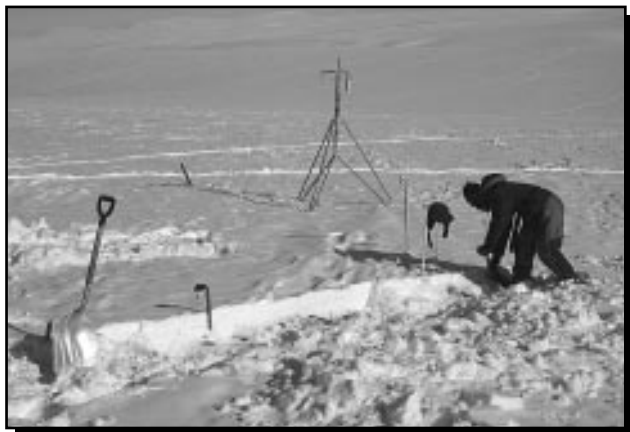
Matthew Sturm digging a trench in March 1992 to examine the micro-topographic variations in the snow and to relate the snow properties to individual tussocks. In the background is a tower with a sonic sounder that recorded the snow depth hourly through the winter, indicating periods of snow accumulation and erosion. (Photo courtesy of Matthew Sturm)
