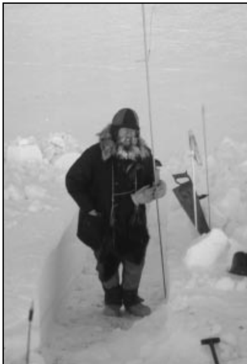
Jon Holmgren, in December 1994, cutting a trench in a large snow drift at Imnavait Creek to expose the snow stratigraphy and to sample for thermal conductivity measurements and density. There is an increasing need for winter access to the TFS area and for winterized living facilities for researchers. (Photo by Matthew Sturm)
