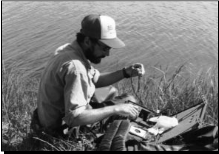
George Kling measuring pH and conductivity and taking samples for dissolved gases in a small tundra stream near TFS in the summer of 1994. (Photo courtesy of Mike Abels)
