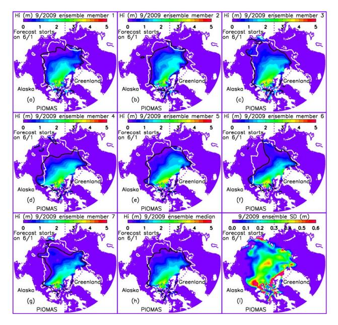
**Figure 3**. September 2009 sea ice thickness predicted by seven individual ensemble members, ensemble median ice thickness, and ensemble standard deviation (SD) of ice thickness. The spatial ensemble median ice thickness distribution (Figure 3h, the same as Figure 2) is most likely to occur in September 2009.
