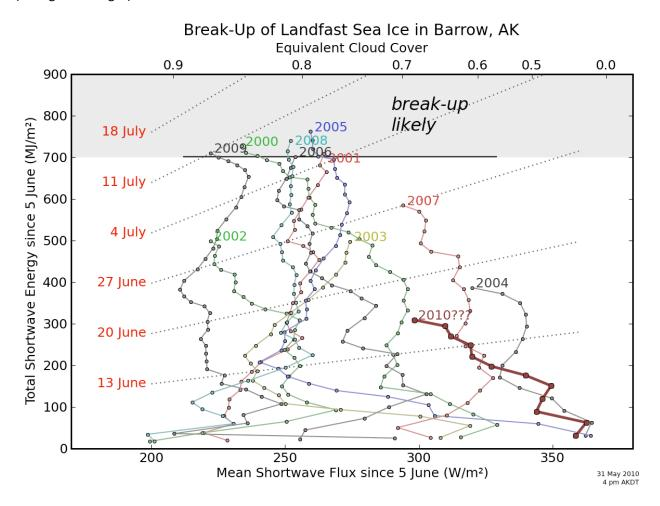
The current 16-day weather forecast does not reach far enough into the future to allow us to project a specific break-up date. In the plot above, the trajectories of incident cumulative solar energy are plotted until break-up for previous years. 2002, 2003, 2004, and 2007 were marked by an absence of grounded, stabilizing pressure ridges. The line marked "2010???" is entirely based on weather prediction at the time of writing. We expect specific break-up forecasts for the second half of June.
