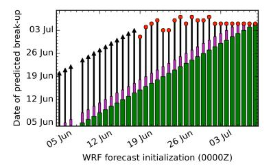
Forecast break-up date (red dots) based on insolation measurements (wide, green bars), estimates based on cloud observations (narrow, purple bars), and weather forecast (black lines). Black triangles indicate that break-up was expected beyond the reach of the forecast. Only break-up forecasts based on 00:00Z weather forecast runs are shown.
